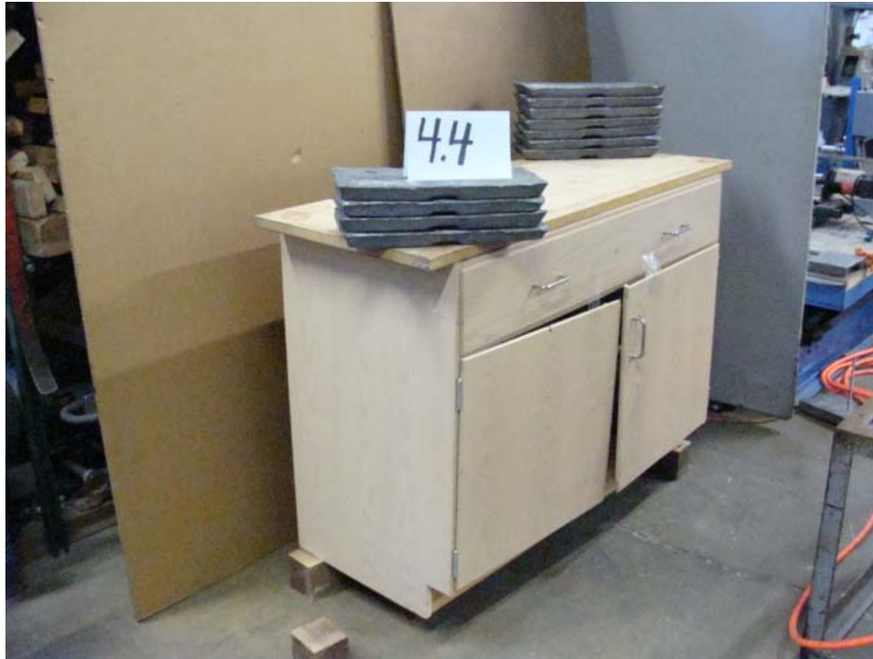
Photo 3: 4.4 Cabinet Torsion Test
