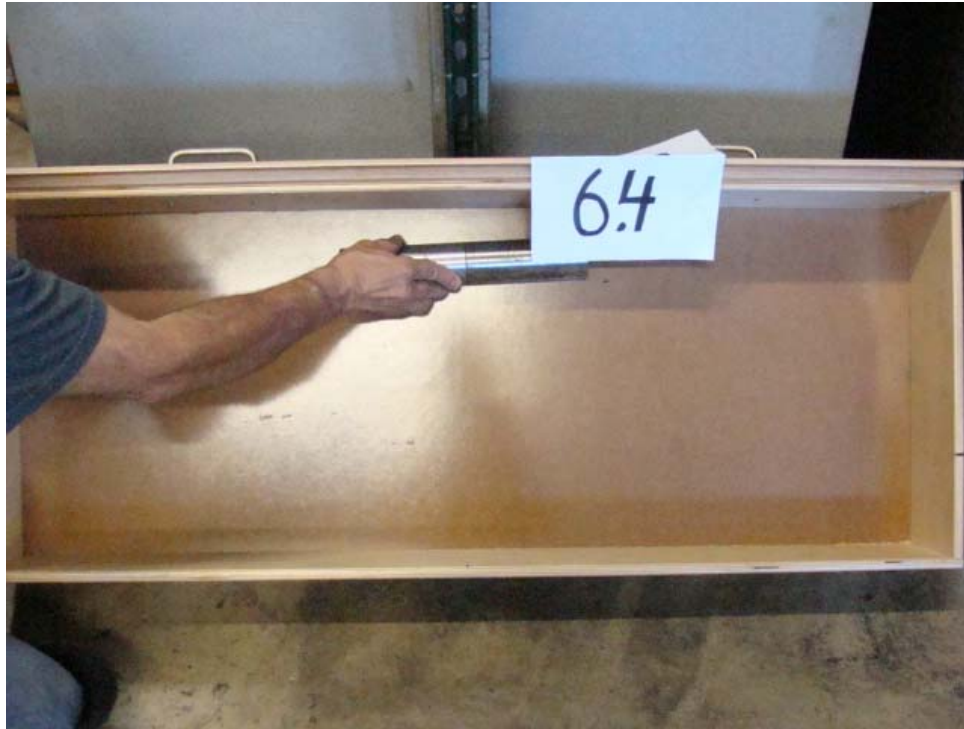
Photo 9: 6.4 Drawer Internal Rolling Impact
