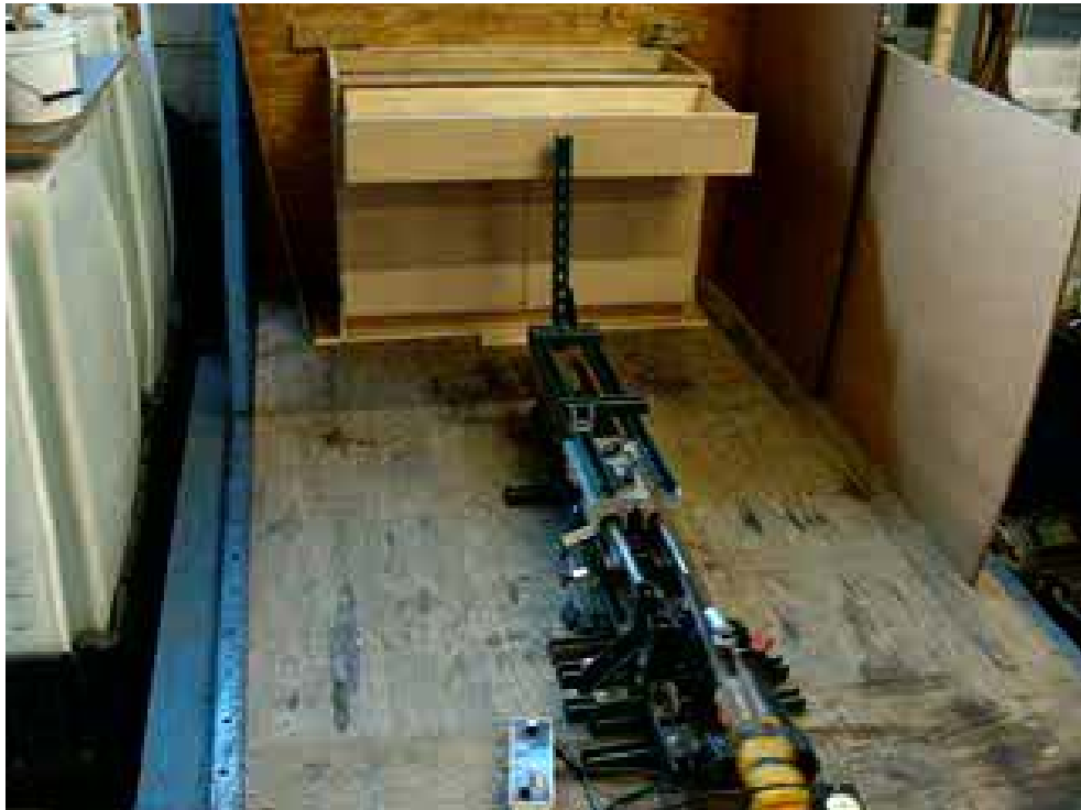
Photo 10: 6.5 Drawer Cycle Test
