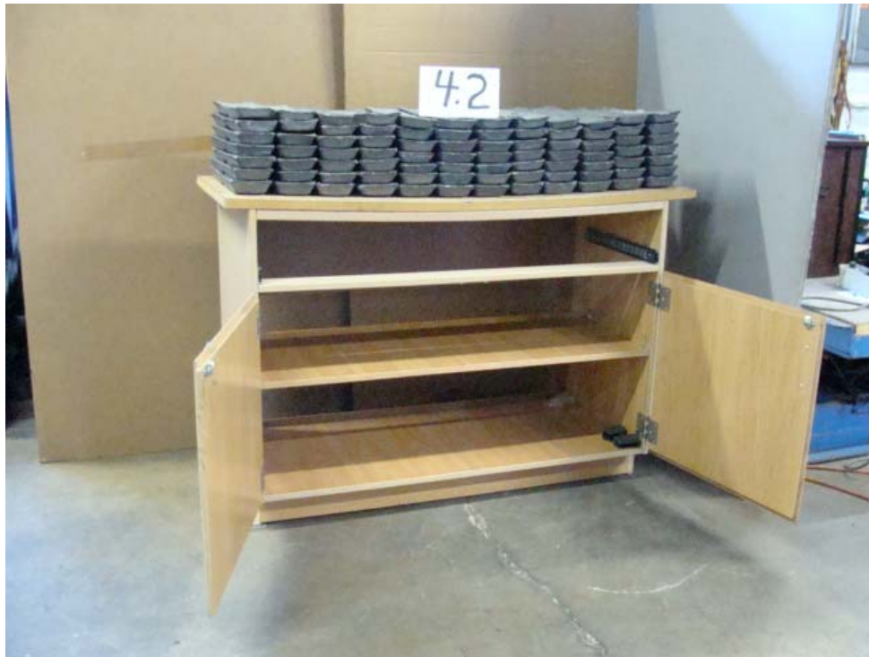
Photo 1: 4.2 Cabinet Load Test
