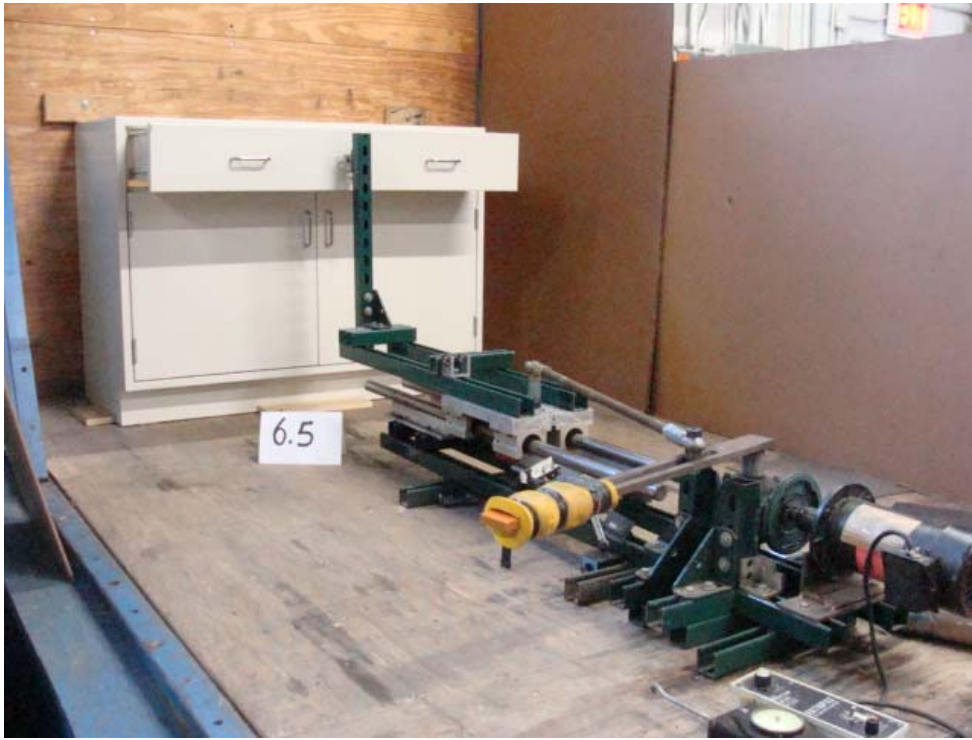
Photo 11: 6.5 Drawer Cycle Test
