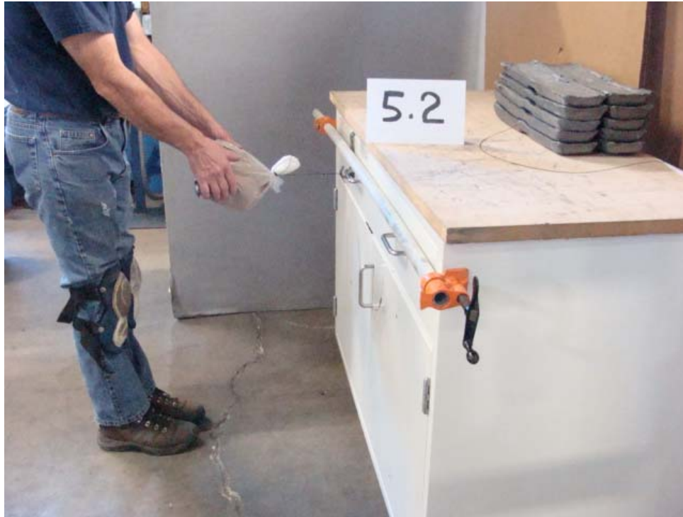
Photo 5: 5.2 Door Impact Test
