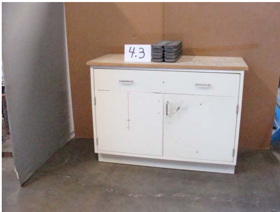
Photo 2: 4.3 Cabinet Concentrated Load Test
