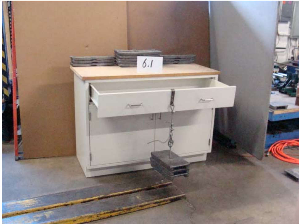
Photo 7: 6.1 Drawer Static Test
