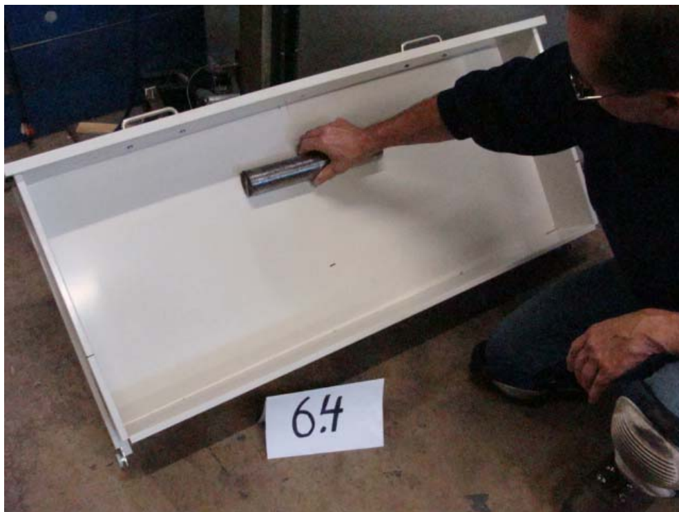
Photo 10: 6.4 Drawer Internal Impact Test
