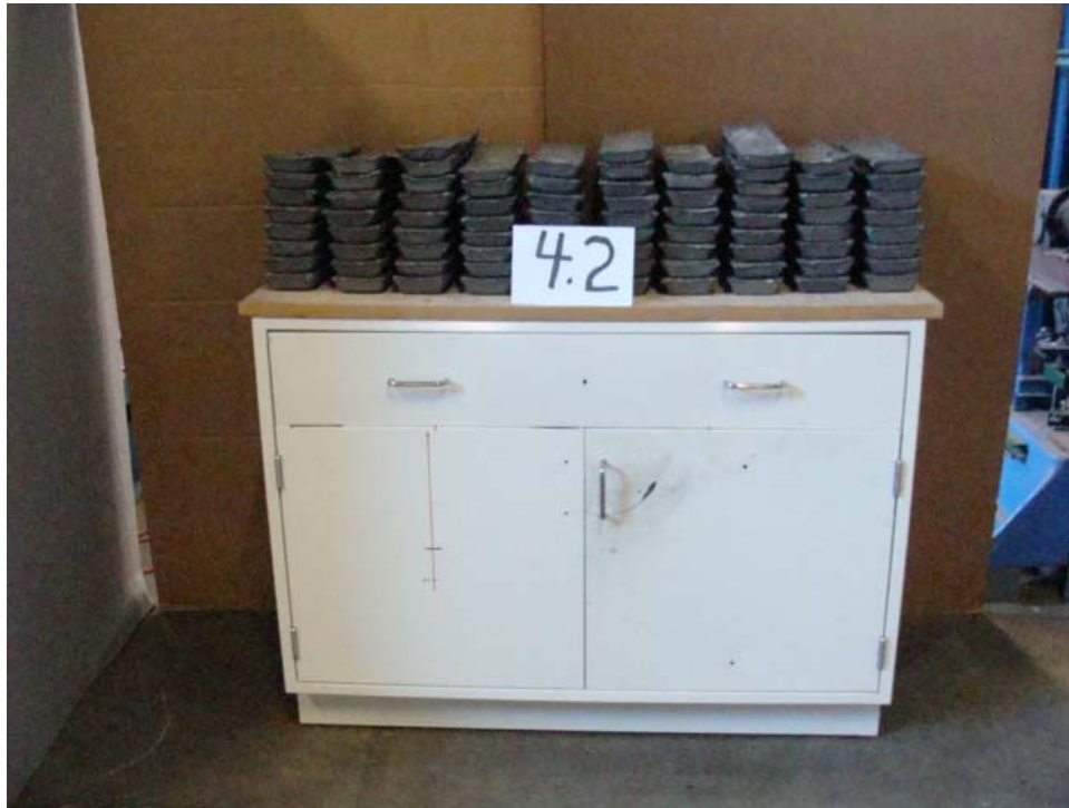
Photo 1: 4.2 Cabinet Load Test
