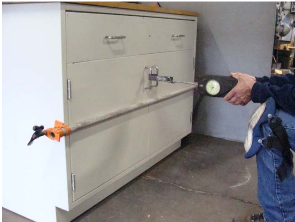
Photo 8: 6.2 Drawer and Door Pull Test
