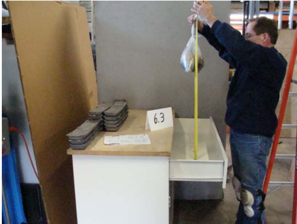
Photo 9: 6.3 Drawer Impact Test
