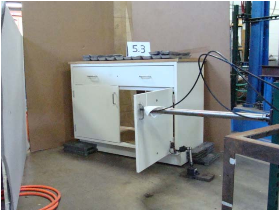
Photo 6: 5.3 Door Cycle Test
